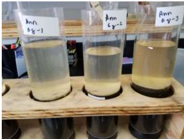
Figure 3. Addition of Phoslock® to sediment incubation systems.
