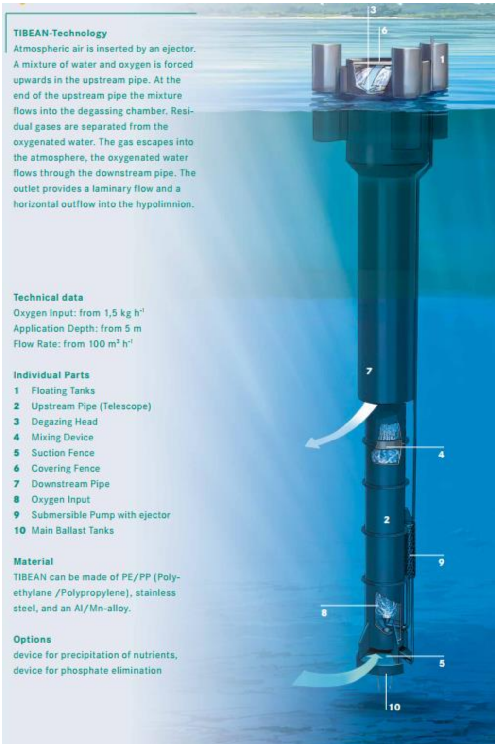
Figure 4-4. Hypolimnetic aeration unit proposed for Ann Lake. Image provided by Canadian pond (Source: www.canadianpond.ca ).
