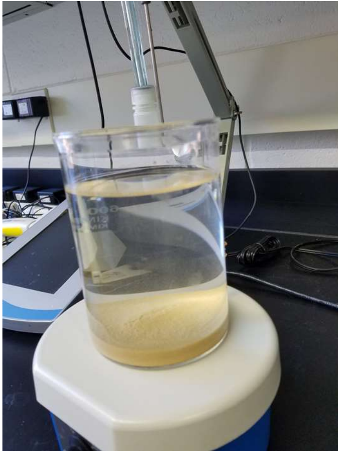
Figure 2. Picture showing the settled Phoslock® slurry.
